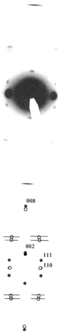
Figure 7. (a, top) Electron diffraction pattern recorded with a tilt angle of 35^\circ (the tilt axis corresponds to the PTFE chain axis) of an oriented PEEK film. (b, bottom) Indexation of the composite electron diffraction pattern: (●) PEEK reflections; (○) PTFE reflections.
