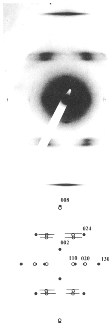
Figure 6. (a, top) Electron diffraction pattern recorded at normal incidence of an oriented PEEK film. (b, bottom) Indexation of the composite electron diffraction pattern: (●) PEEK reflections; (○) PTFE reflections.
